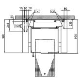
**Electric** Supply voltage: 400 V/3N ph/50/60 Hz Total Watts: 15.5 kW Installation: FS on concrete base;FS on feet;On base;Standing
